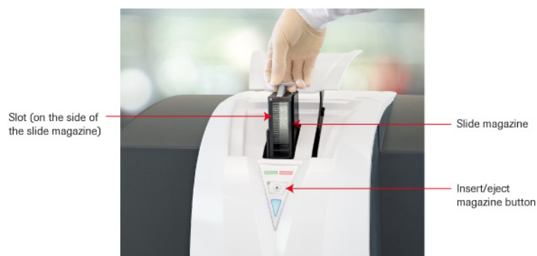
Figure 13: Inserting the Slide Magazine into the Scanner
